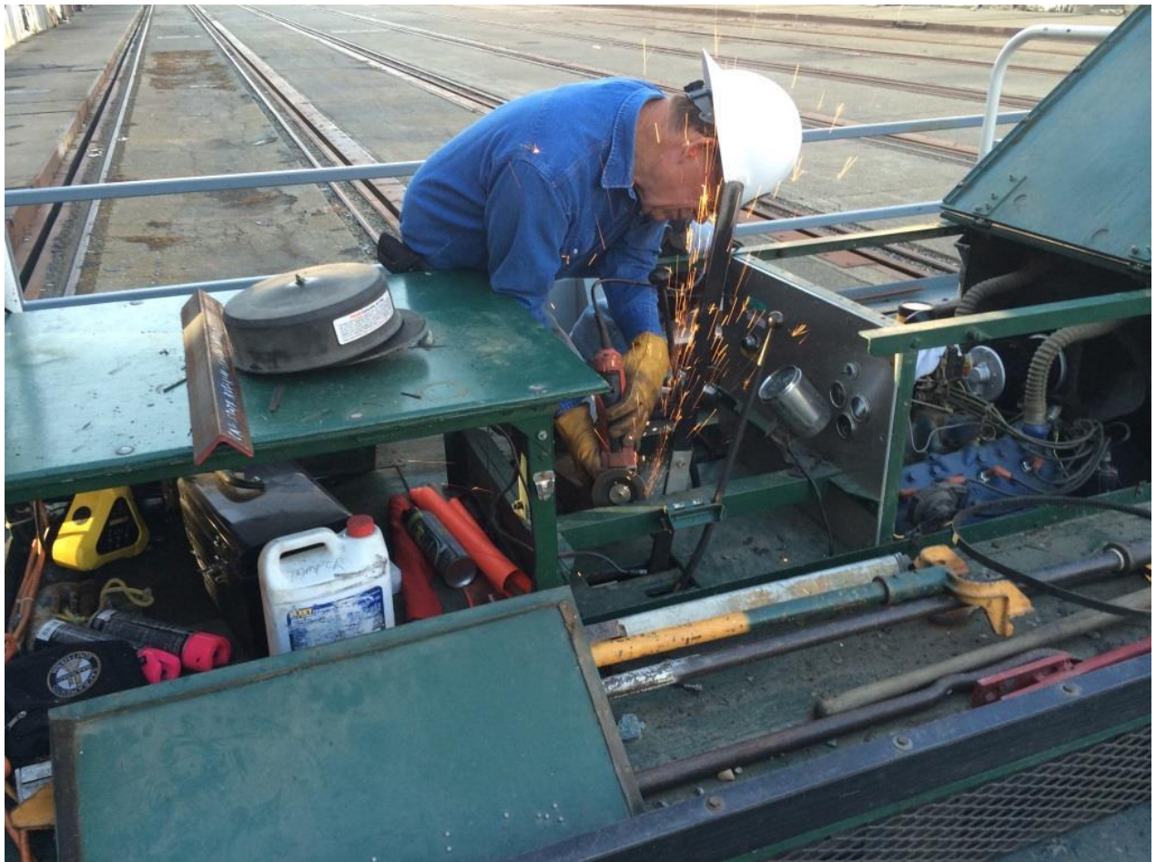
Cliff grinds new notches into the cross-piece that holds the brake lever in position when set
